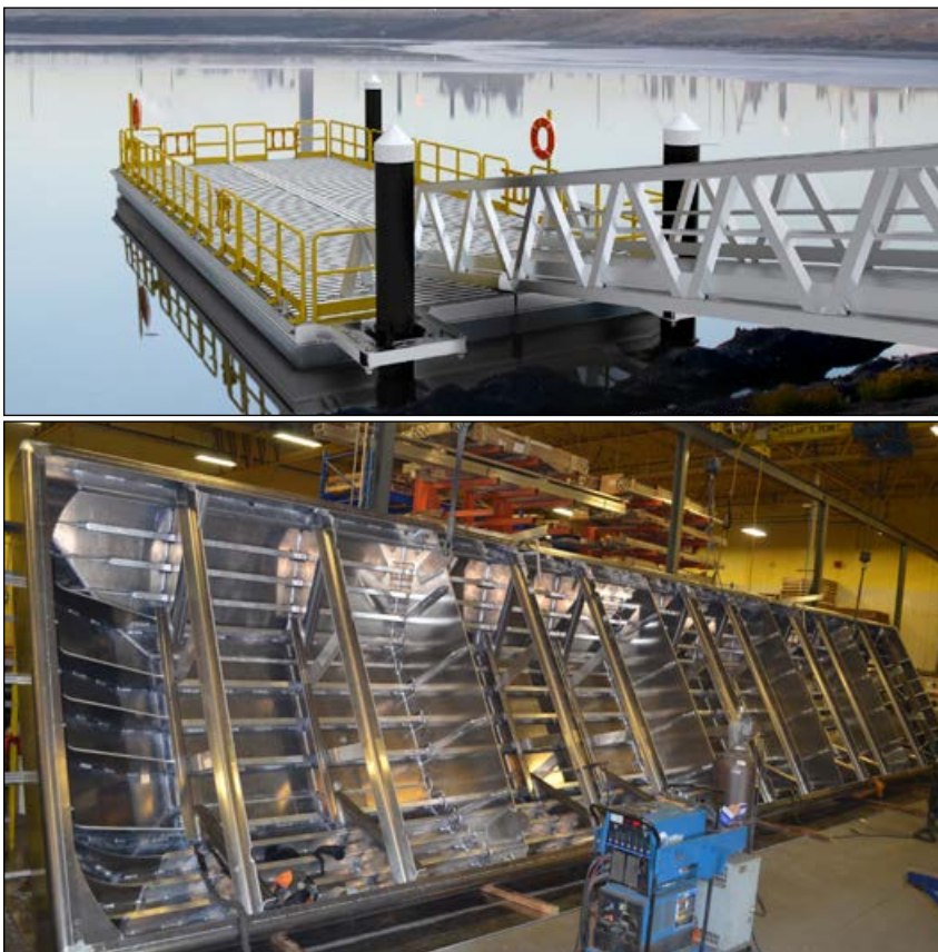
Figure 3. Top: Rendering of aluminum barge MAADI designed and built in October 2012. 5083 plate was used for the hull of the structure during the construction process and marine bulbs were extruded from 6061 T6 alloy. Bottom: The internal structure of the port side of the barge is shown. The structural arrangement sustains the pressure of one meter of ice thickness.
